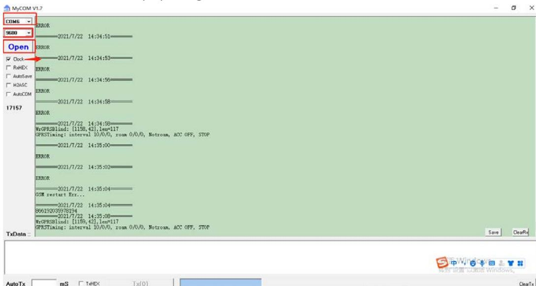
**Format to send command to the device through MyCOM software**
