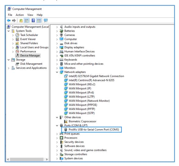
Run parameter tool, choose "COM3" port, "9600" baud rate, and click "Open" to open the port.
