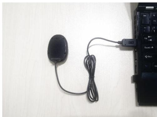
Connect device to PC with **configuration data cable** (optional accessory). Run “fifotrack Parameter Tool” software, choose correct port, always select 9600 baud rate, click “open” button.
